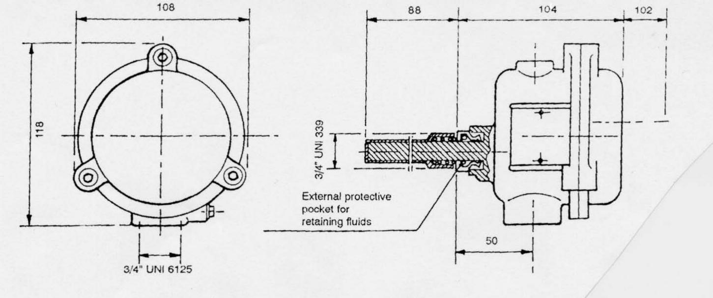
B = minimum space necessary for removing the housing without unscrewing the sheath. This design allows rapid replacement of the monitoring equipment without the need for emptying installations or tanks.
